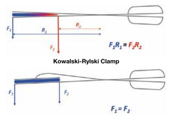
Figure 1. Stress distribution along the clamp jaws. In currently available clamps according to the law of the lever, the aortic area near the hinge is under more stress (F2) than the aortic area distal to the hinge (F1). In the novel Kowalski–Rylski clamp an additional hinge allows the upper jaw to adjust its position according to the pressure resulting in equal pressure distribution along the jaws.
