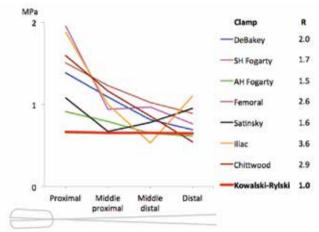
Figure 2. Maximal clamping pressure generated at proximal, middle proximal, middle distal and distal areas to the clamp hinge quartiles. The proximal quartile is near, the distal quartile far from the clamp hinge. R – ratio between the highest and lowest pressure measured along the clamp jaws; SH – straight handle; AH – angled handle.
